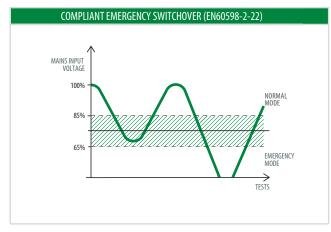
When mains power dips the emergency must turn on at the correct voltage.
